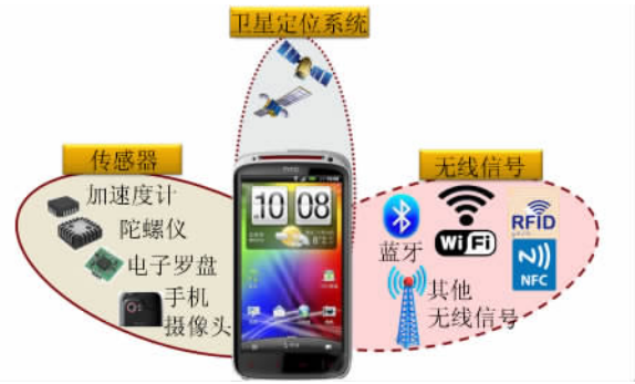
图 4 基于多传感器多网络的位置服务 Fig. 4 Location Service Based on Multi-sensor & Multi-network
