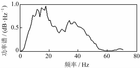
图 5 低通滤波后噪声的功率谱密度 Fig. 5 Power Spectrum Density of Noise After Low-Pass Filtering
