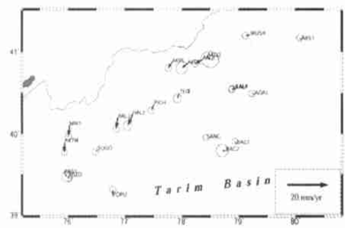
图4 去掉塔里木块体整体运动后(欧拉矢量)的测站速率残差矢量 Fig.4 Residual Vectors Between the Euler Vector Predicted and GPS Determined Velocity Vectors
