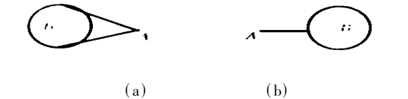
图3 4元组空间关系描述框架 area/line 情况不能区分示例 Fig. 3 The Example with the Same Value Under 4-intersection Model
