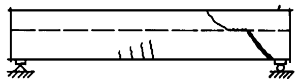
Fig. 4 Failure Modes for Reinforced Concrete Composite Beams without Stirrups
