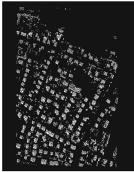
图 2 通过高程阈值获取的建筑点 Fig. 2 Building Points Gained by Threshold of Height
