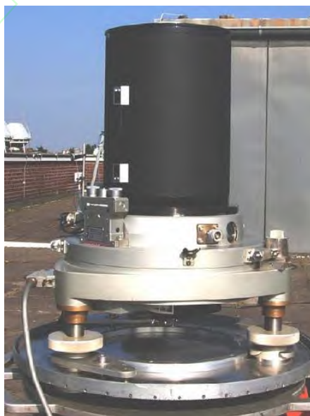
Fig. 4 TZK2-D digital zenith camera system [18]
