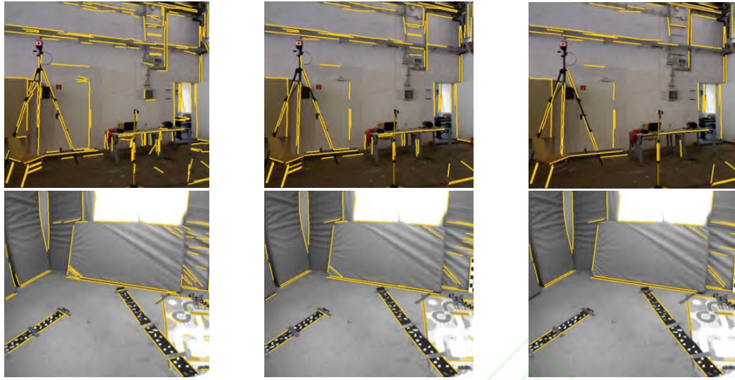
Length:20 pixel Length:30 pixel Length:40 pixel 图 7 不同长度阈值条件下的线特征提取结果 Fig.7 The Line feature Extraction Results under Different Length Thresholds Conditions
