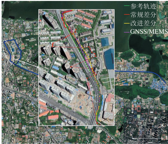
图 14 高架遮挡场景下 3 种处理策略的轨迹对比 Fig. 14 Track Comparison of Three Different Positioning Strategies Under Viaduct Occlusion Conditions
