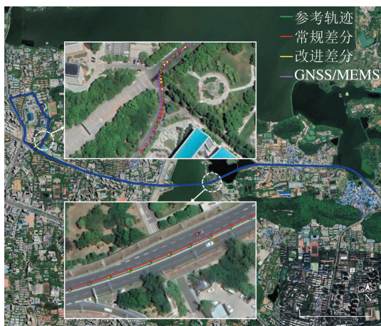
图10 开阔天空场景下3种处理策略的轨迹对比 Fig. 10 Track Comparison of Three Different Positioning Strategies Under Open Sky Conditions
