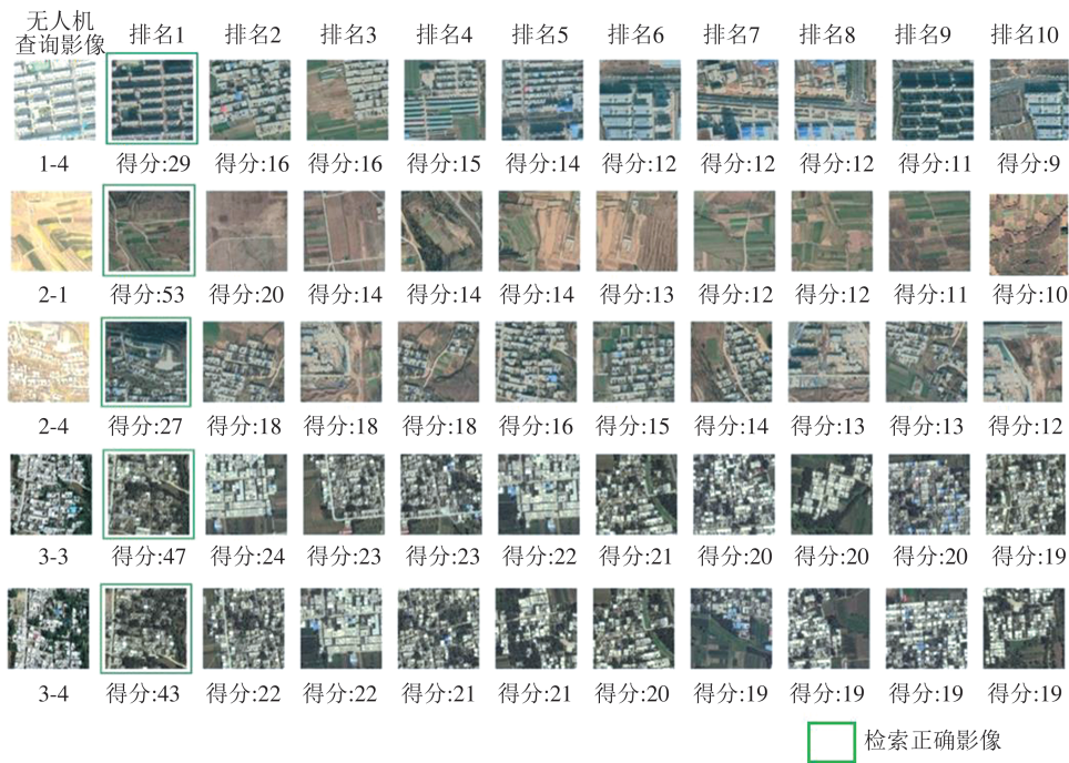
图 12 无人机视频影像检索精匹配重排序后结果 Fig.12 Unmanned Aerial Vehicle Video Image Retrieval Results After Precise Matching and Reranking
