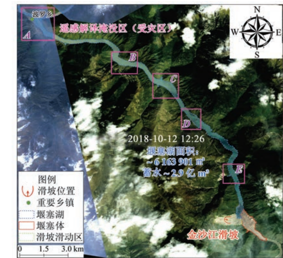
图 8 金沙江首次滑坡淹没区分析 Fig. 8 Analysis of the Inundated Area of the First Jinsha River Landslide
