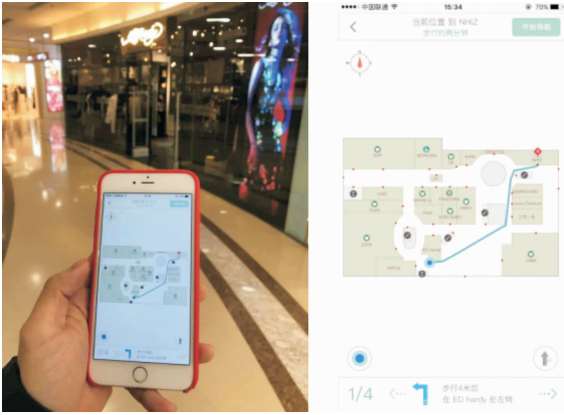
图 15 基于通行区域模型的室内路径实时规划及表达 Fig. 15 Indoor Route Real-Time Planning and Presentation Based on Traversable Region Model
