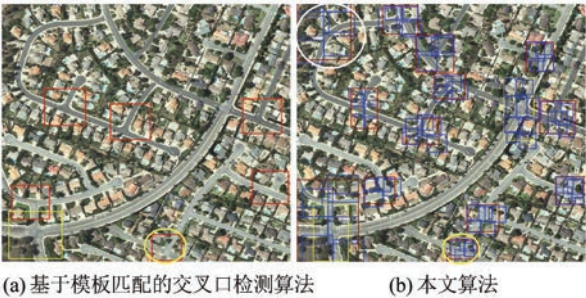
图3 法国巴黎城区 2 m 分辨率 GeoEye-1 遥感影像道路交叉口检测效果示意图 Fig.3 Detection Results of Road Intersection on 2 m Resolution GeoEye-1 Images for Paris, France
