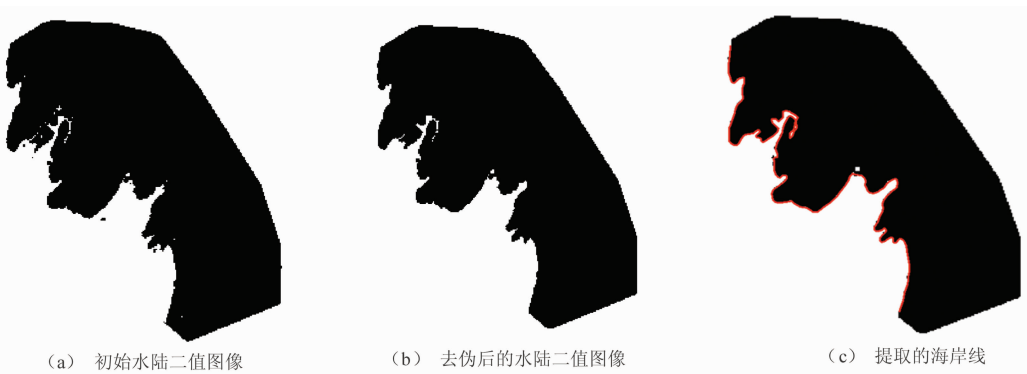
图 3 二值图像改进法提取海岸线 Fig. 3 Improved Binary Image Method to Extract Shoreline
